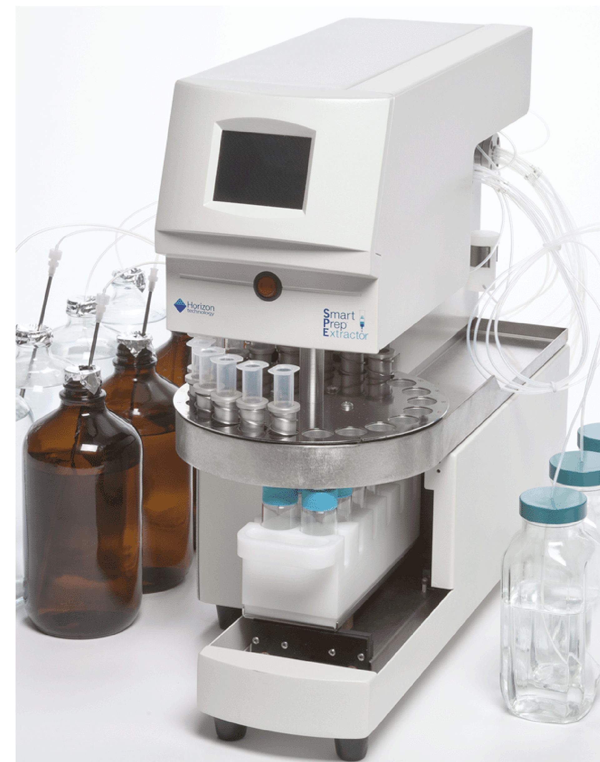
Figure 1: SmartPrep™ - Automated solid-phase extraction system by Horizon Technology for sample processing of Echinacea preparation
